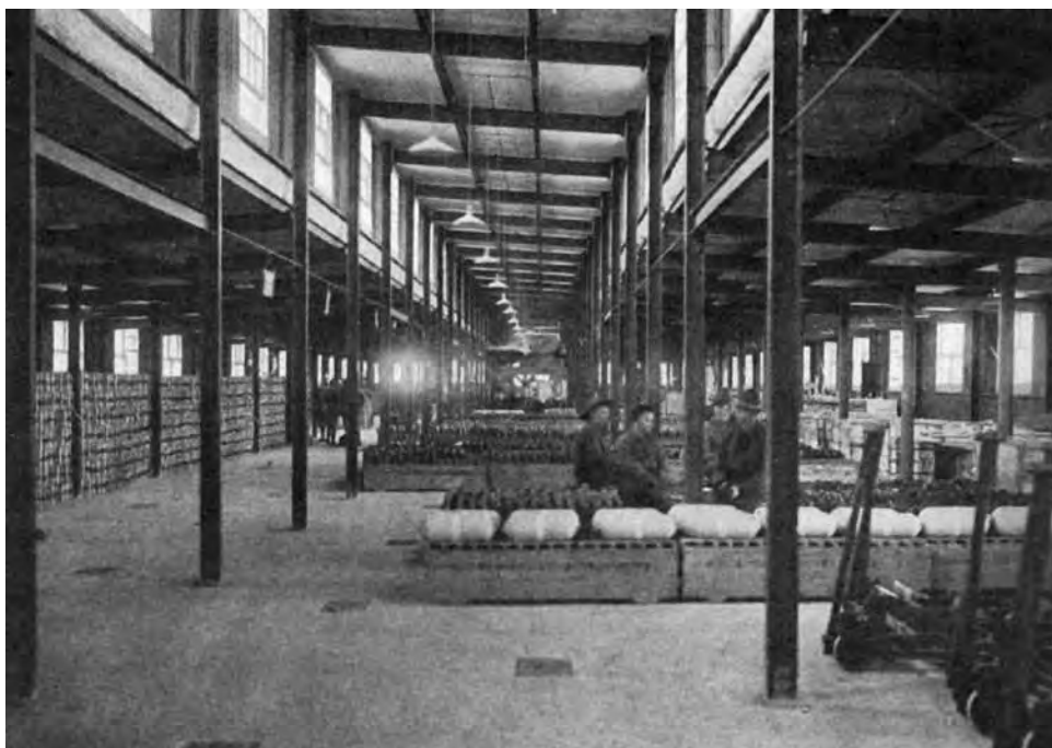
Filling drums with phosgene and, in storage, performing a leakage test
