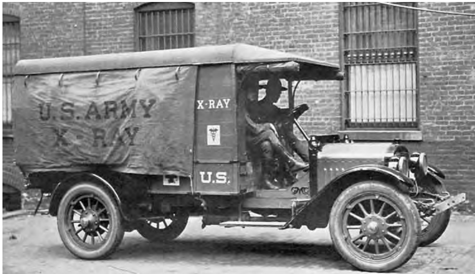
General Motors-built truck retrofitted to carry X-ray equipment; (below) mobile delousing unit
